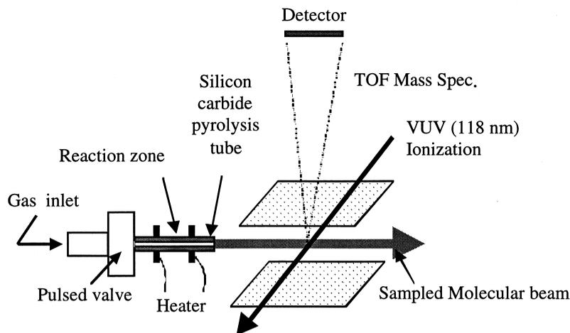
Fig. 1. Schematic of the pyrolysis/supersonic jet expansion/photoionization/time-of-flight mass spectrometer apparatus used to observe thermal decomposition products.
