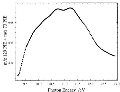
Fig. 4. Fragment ion intensity ratio of M- $\text{CH}_3$  ( $m/z$  129) to M- $\text{C}_5\text{H}_{11}$  ( $m/z$  73) ions from photoionization of room temperature  $(\text{CH}_3)_3\text{CCH}_2\text{C}(\text{CH}_3)_2\text{OCH}_3$  (TOME) as a function of ionizing energy. The PIE ratio curve was fitted using 20-point FFT smoothing.
