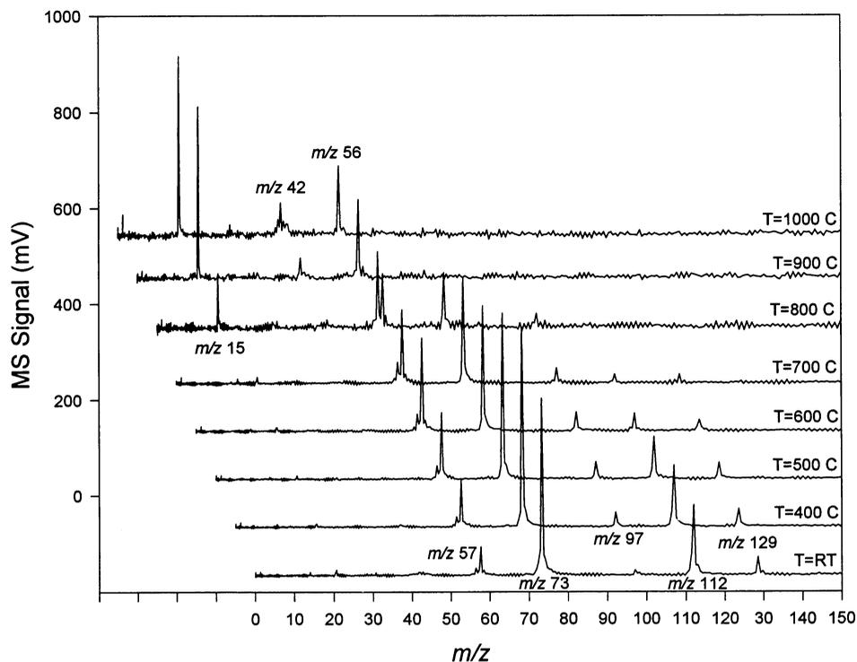
Fig. 5. Stack plot of pyrolysis/supersonic jet expansion/118 nm photoionization TOF mass spectra of TOME as a function of nominal temperature. Nozzle temperature is related to the nominal temperature by the empirical expression given in Sec. 2. Peaks from the expansion gas (argon) have been subtracted.
