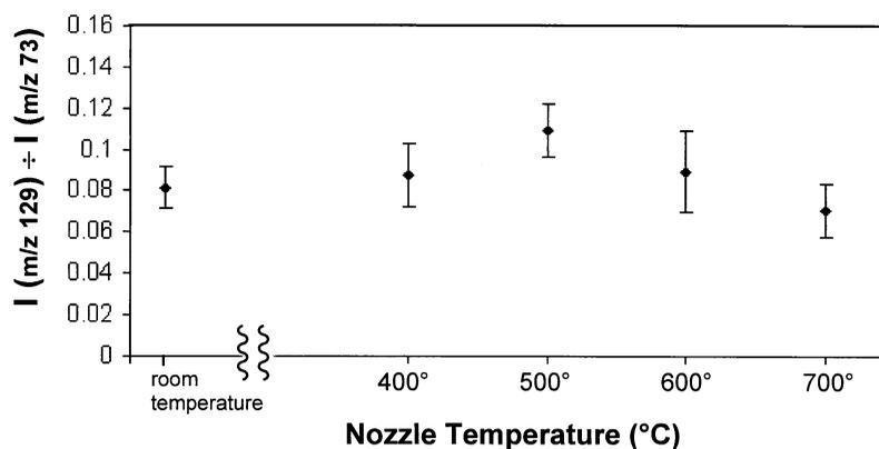
Fig. 6.  $[M-CH_3]:[M-C_3H_{11}]$  ion intensity ratio for pyrolysis/supersonic jet/118 nm photoionization TOF mass spectra of TOME as a function of nominal temperature, showing no significant variation. Nozzle temperature is related to the nominal temperature by the empirical expression given in Sec. 2. Error bars stand for sample standard deviations.
