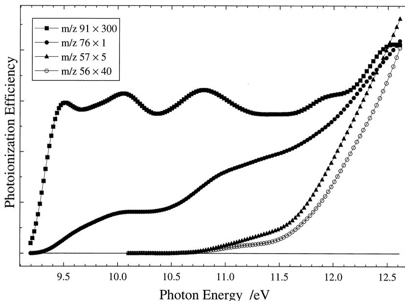
Fig. 2. Photoionization efficiency (PIE) as a function of wavelength for room temperature  $(\text{CH}_3)_3\text{COCD}_3$  (MTBE- $d_3$ ) as a function of ionizing energy. The PIE curve was fitted using 15-point FFT smoothing.
