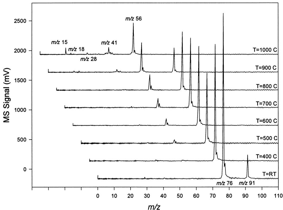
Fig. 3. Stack plot of pyrolysis/supersonic jet expansion/118 nm photoionization TOF mass spectra of MTBE- $d_3$  as a function of nominal temperature. Nozzle temperature is related to the nominal temperature by the empirical expression given in Sec. 2. Peaks from the expansion gas (argon) have been subtracted.
