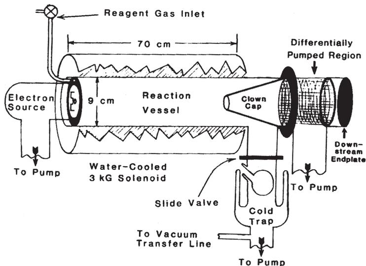
**Figure 3.** Schematic of an Electron Bombardment Flow (EBFlow) reactor. The magnetic field maintains the electron beam along the axis of the solenoid. The beam's negative charge prevents cations from migrating to the walls, and all charged species are dumped into the differentially pumped region downstream of the clown cap, where they are pumped away and do not contaminate the neutrals collected in the cold trap, which come from the EBFlow reaction vessel.
